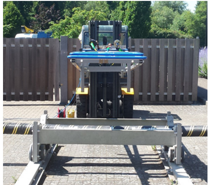
The Target Scaling procedure involves the use of a 'factory calibrated system' and a customer supplied real sample (4 – 5m in length) of the target to be surveyed.
